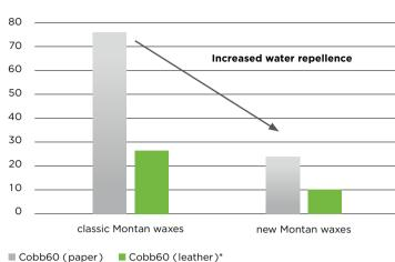
**Cobb60** [g/m<sup>2</sup> min]: Water adsorbed by the coated surface during 60 s contact. \*For leather, the Cobb60 measurements were performed after application of mechanical stress on the coated surface.
