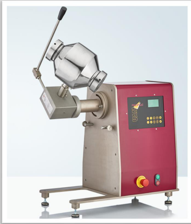
Double cone blender for powder /granulation blending
