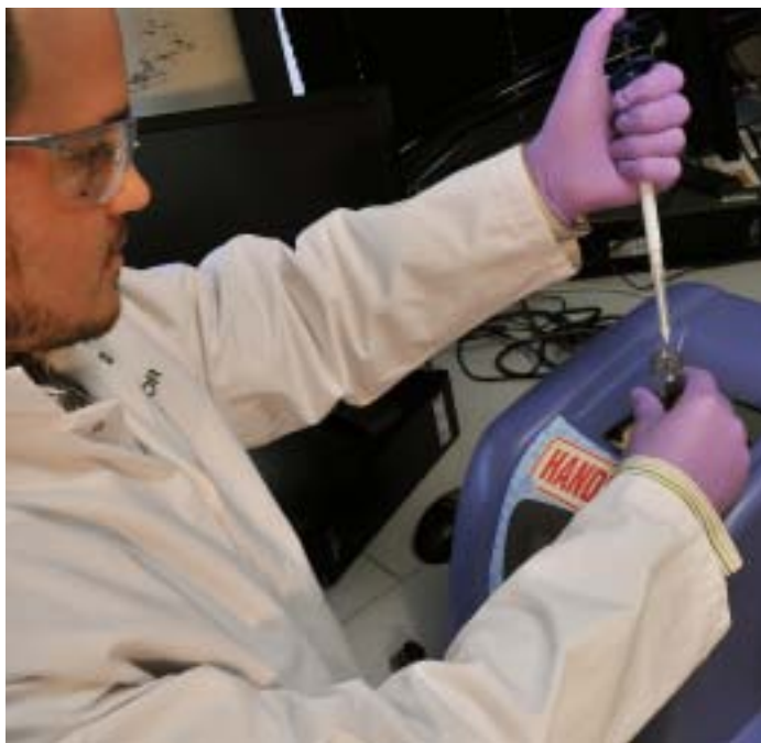
TESTING TIMES: At the Clariant laboratory in The Woodlands, Texas, a laser dispersion tester is used to determine the efficacy of asphaltene inhibitor chemistries.
