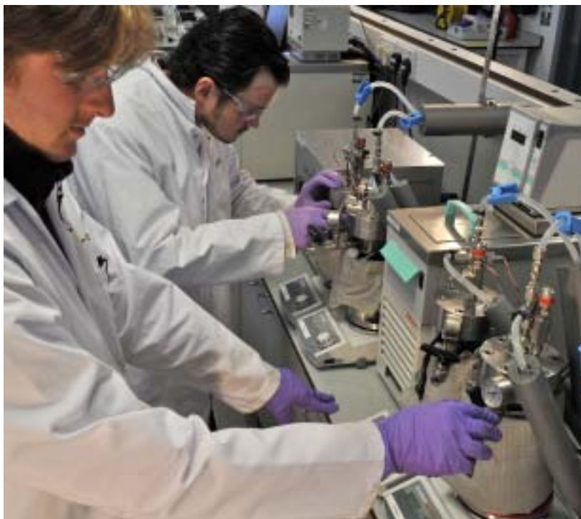
WAX WORKS: Testing wax inhibitor products on coaxial shear testing units.
