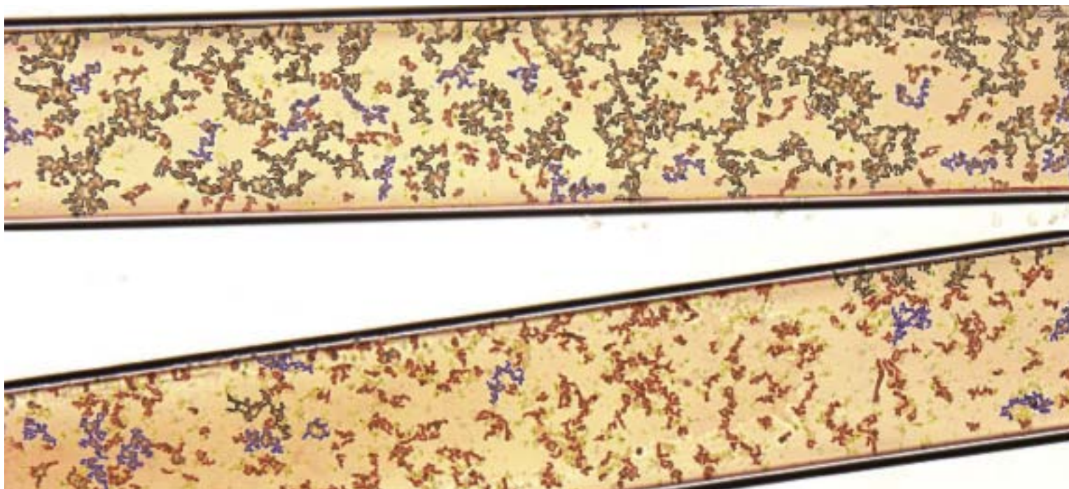
CAPILLARY ACTION: Image shows the raw output of a microscopy technique in which Clariant precipitates asphaltene crystals in a capillary, and the software colours them and counts them, making it a quantitative method. The top capillary is untreated, while the bottom capillary is treated.
