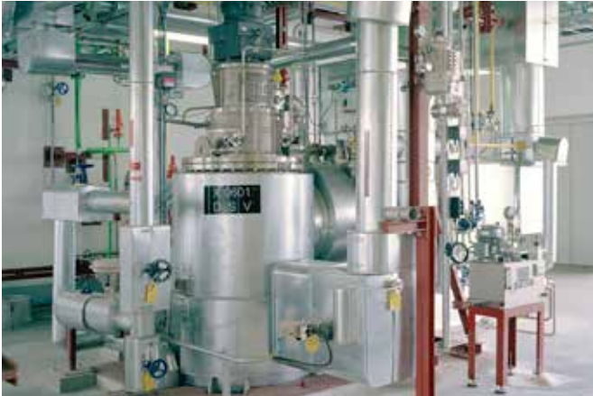
Distillation unit in Clariant's Licocene wax manufacturing Destillationsanlage in der Fertigung der Clariant Licocene Wachs
